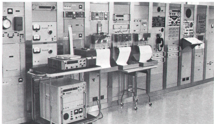
Dominion Observatory at Ottawa, Canada, is one of major time-keeping centers which compared time with flying clock (below table).
