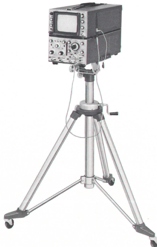
Fig. 16. New, lightweight scope cart is patterned after a camera tripod and has adjustments for tilt and height.
